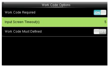
When you turn **ON** the workcode required it will ask you to set the timeout for the input screen.
