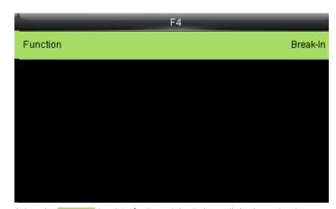
Select the **Function** Break-In for F4 and the F4 key will display as Break-In on the main screen.
