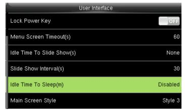
This parameter is used to specify a period after which the device is put in sleep mode if no operation within this period. You can wake up the device from sleep by pressing any key or touching the screen.
