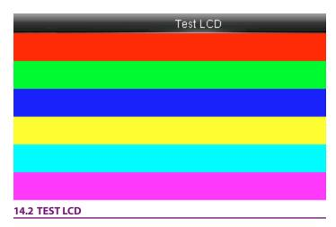
The terminal automatically tests the display effect of the color TFT display by displaying full color, pure white and pure black and checks whether the screen displays properly.
