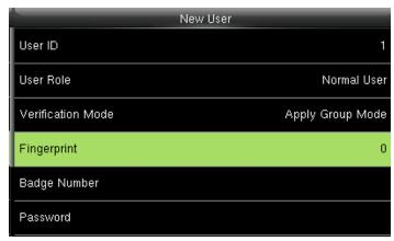
To enroll the fingerprint for the new user select **fingerprint** .
