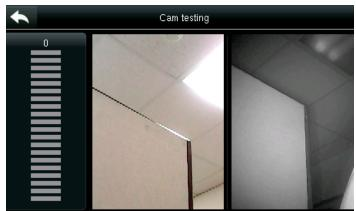
When you select to test the face the above image will be displayed where you can put your face and verify whether the cam is working properly.
