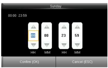
Press / to select a time option and press  $\checkmark$  /  $\blacktriangle$  to set time. After setting a period of time, press  $\overline{OK}$  to save the setting and exit
