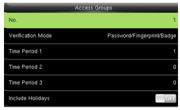
The No. cannot be modified, and the other operations are similar to those performed to add a new group. Press left arrow on the screen to return
