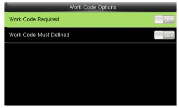
When the work code required is **OFF** it will disbale the required work code.
