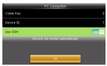
When you turn **ON** the "SSH" function the device will restart automatically as shown above.
