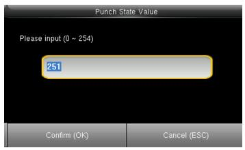
You can change the value of the punch state by changing the value in the input screen with the help of keypad.
