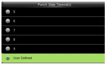
You can change the punch state timeout from the image above. The timeout ranges from 5 to 99 sec.
