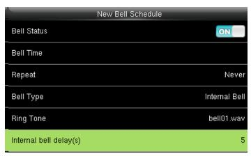
Select Internal bell delay (s) and press OK. It specifies the duration for ringtone playing.
