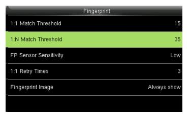
Here select 1:N match threshold The value is similar to verification and the enrolled template.
