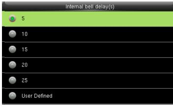
You can edit the delay of the internal bell from the image above. It ranges from 5 to 99 seconds.
