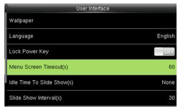
The device will display the main interface automatically when no operation is performed on a menu within the menu timeout time
