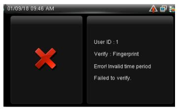
A user punches in off the activate schedules, the device will notify the user by "Error! Invalid time period Failed to verify."
