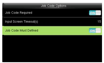
Turning ON options will enable the Job Code Required function Switch "Job Code Must Defined" to ON to force a job code to be selected before verification
