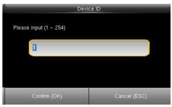
Here you can put the number for this device by using the keypad in the input screen as shown above and press OK.
