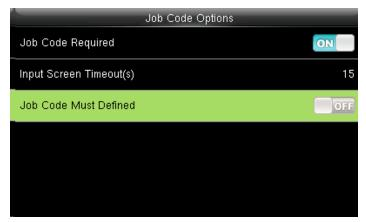
Turning ON options will enable the Job Code Required function Switch Job Code Must Defined to OFF will not force a job code to be selected before verification
