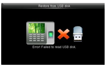
If the USB disk is not properly inserted the above screen will be displayed. You can either change the USB or insert it properly again.
