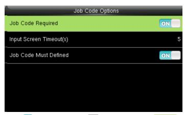
Turning ON options will enable and OFF options will disable the Job Code Required . "Input Screen Timeout(s)" is used to set up the time period for displaying the job code list in seconds.
